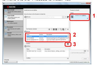
3 Select the utility to be installed, and then click the arrow button to move it to the "Products to Install" list.
