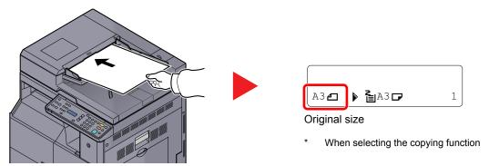
Put the side to be scanned (or the first side of two-sided originals) face-up. Slide the leading edge into the document processor as far as it will go.
